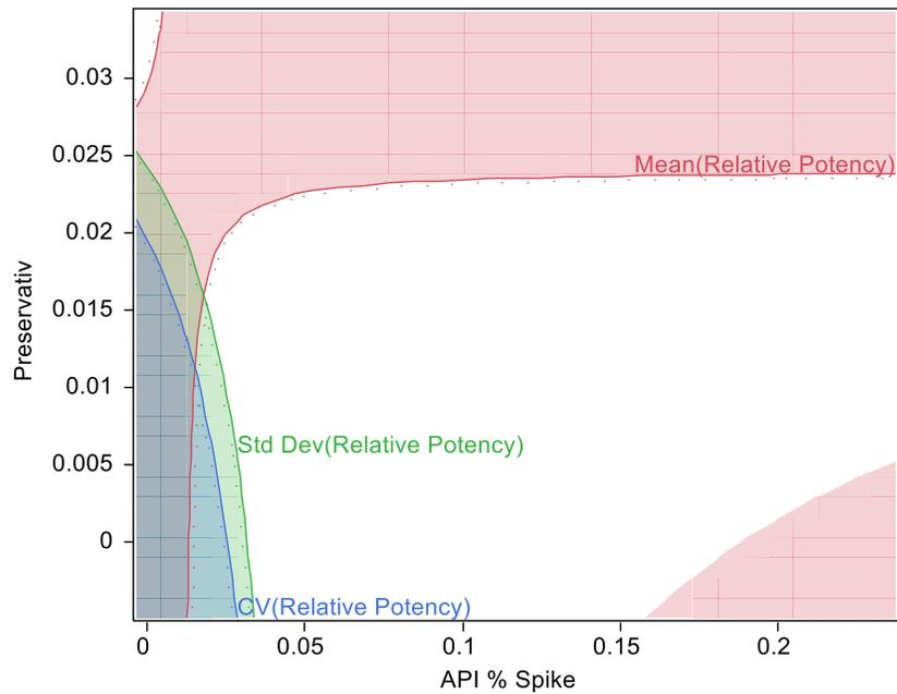
Figure 5. DOE Design Space for Method Precision and Bias
